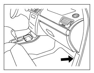
The fuse block is located on the passenger side of the vehicle in the carpet molding. Remove the fuse block door to access the fuses.
